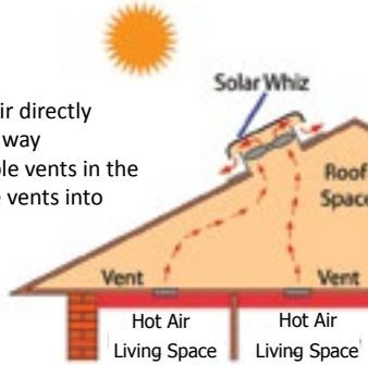
If required, it is possible to connect ducting to the Solar Whiz to extract air from specific areas.
